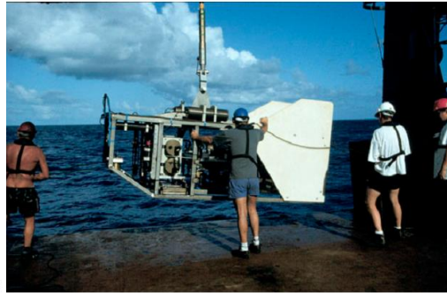
Figure 11: The Southampton Oceanography Centre's deep-tow hydrothermal plume instrument BRIDGET being prepared for launch from the RRS Charles Darwin at the Mid-Atlantic Ridge
