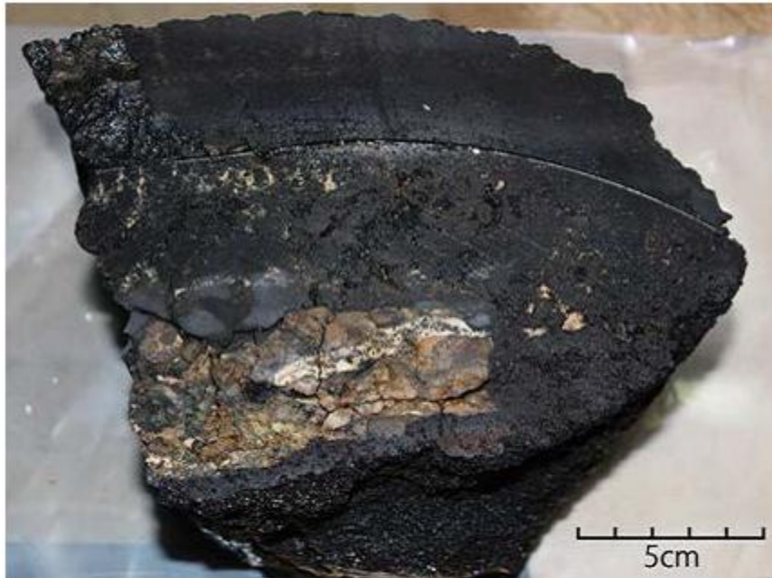
Figure 5. Cross section of a ferromanganese crust collected at the Takuyo Daigo Seamount
